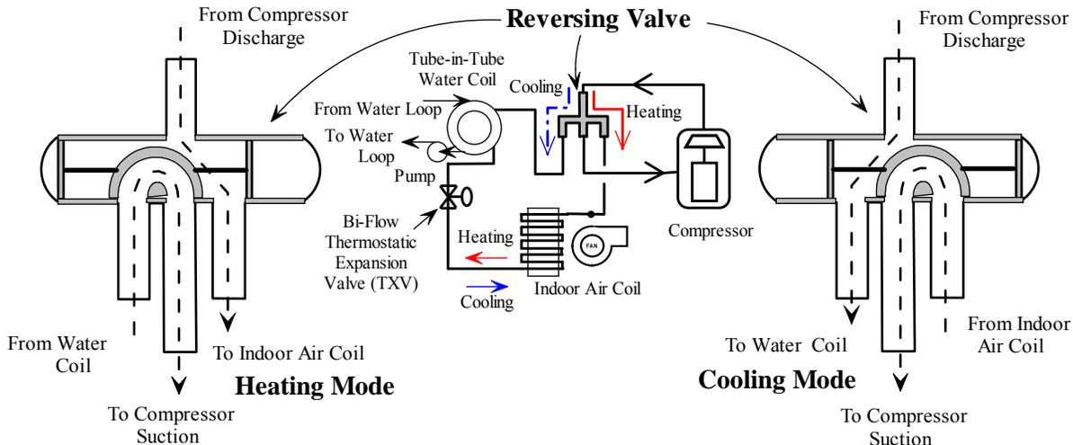
Figure 5. Reversing Valve that Enables an “Air-Conditioner” to be a “Heat Pump”
