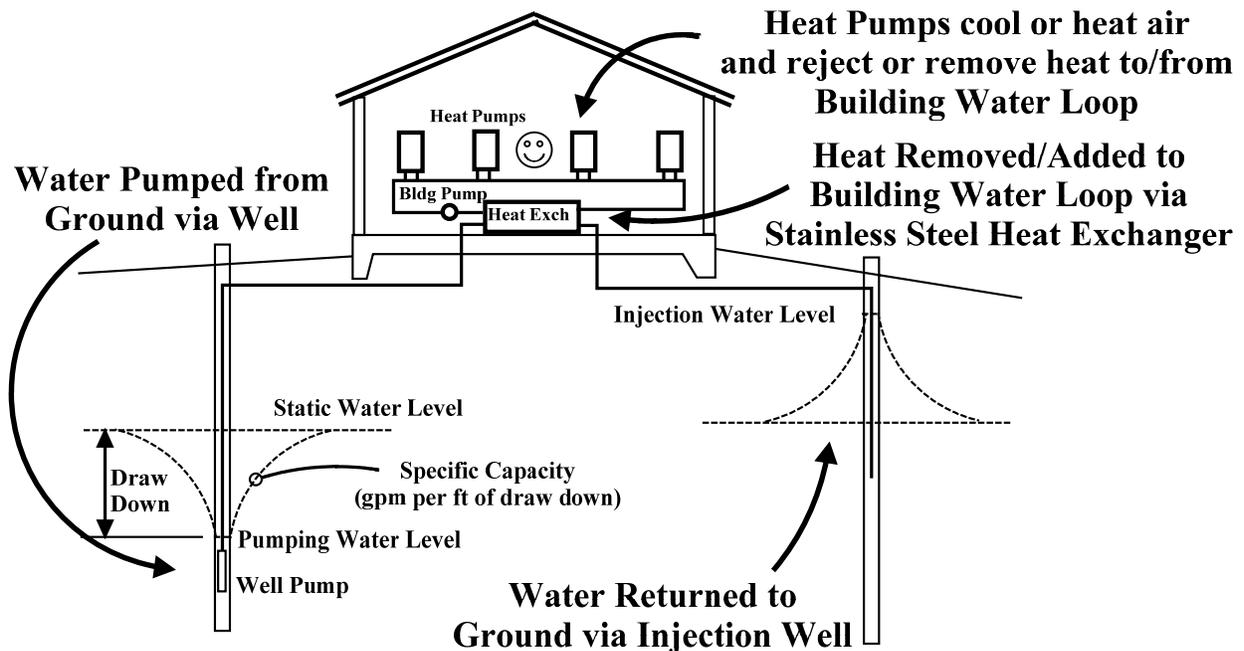
Figure 3 Ground Water Heat Pump System (Open-Loop)
