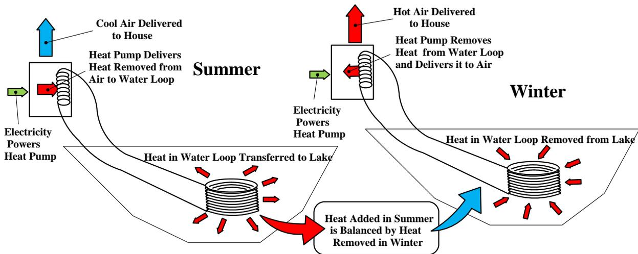
Figure 2. Lake Source Heat Pump (Closed Loop Type)
