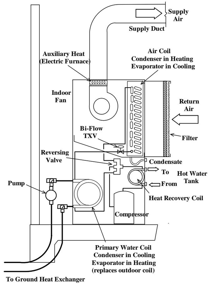
Figure 6. Ground Source “Geothermal” Heat Pump Unit
